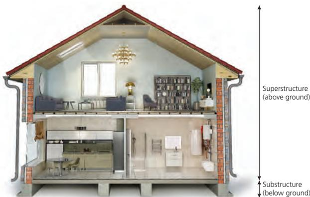
▲ Figure 3.1 Superstructure and substructure of a building
