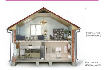
Figure 3.1 Superstructure and substructure of a building By contrast, the substructure of a building is the part below ground level. For more information on superstructure and substructure, see Chapter 7.
