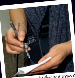
Use tissue to test the flow and pressure through the airbrush.
