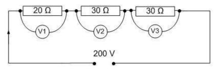
For the circuit shown, what would be the voltage reading of voltmeter (V1)?
