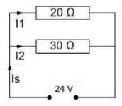
What is the relationship between voltage and current across the resistors for the circuit shown?
