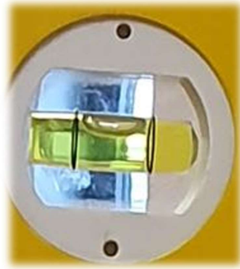
Gothic window installed plumb to the dormer within 0.5mm.
