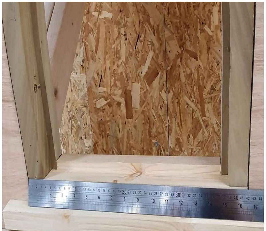
Gothic window within 1mm of the stated width.
