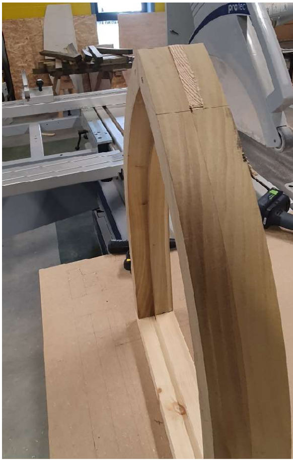
Gothic window loose tenon joint showing accuracy in joints from accurate measuring, marking and cutting of components before dry fitting.
