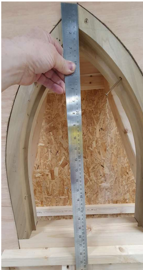
Gothic window height within 1mm of the stated dimension.
