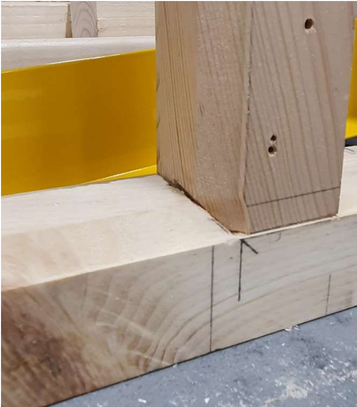
Mitre to rebated mortise and tenon tight within 3mm.
