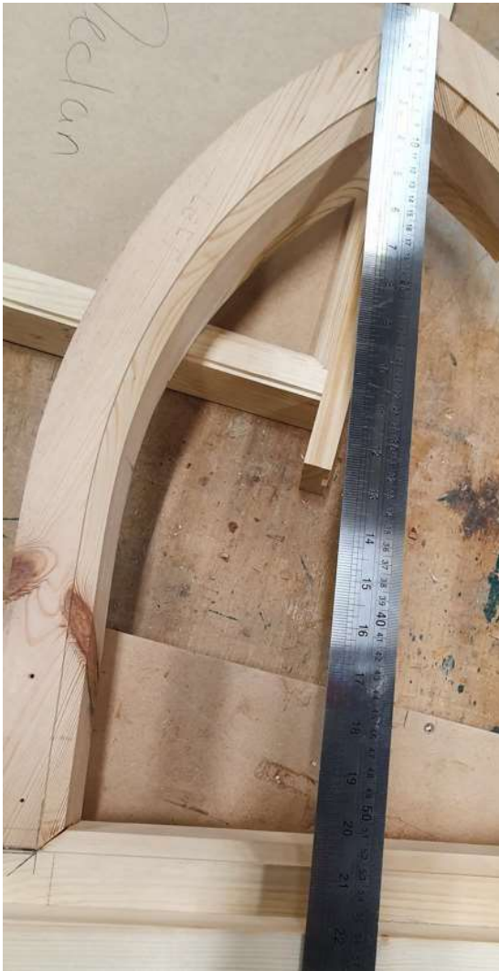
Gothic window height within 3mm of the stated dimension
