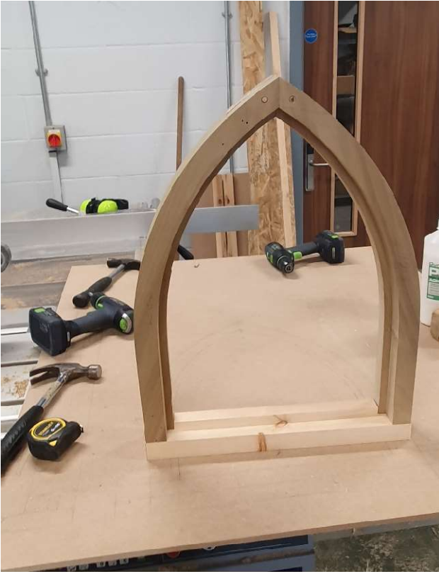
Gothic window assembled pre subsill and assembly working area.
