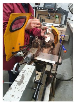
Photograph 21 and 22 – showing in-production accuracy checks being taken. Measuring the internal diameter with a bore mic and the external with an external micrometer.
