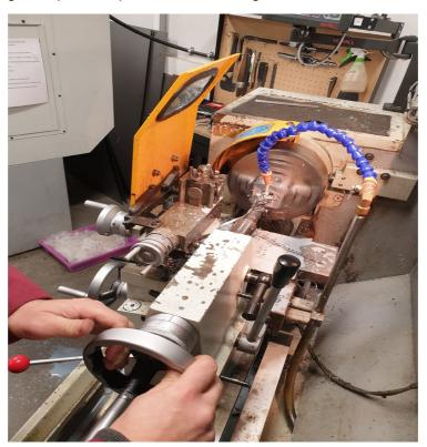
Photographs 17, 18 and 19 – showing the bored out bearing housing until nylon top hat was a push fit. Using the bore micrometer to help get close to the size before using the component as a final fit.
