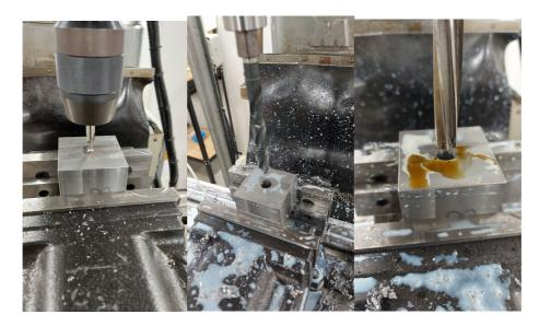
Photographs 14 and 15 – showing a small plug was made that fitted into the 14mm reamed hole, this gave a gauge to get it clocked in centrally, it was then rechecked with the plunger dial test indicator (DTI) on the 4 faces and minor adjustment made to make sure it was central.
