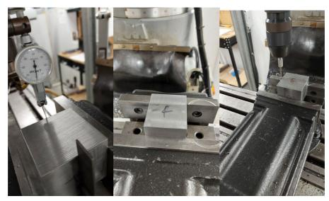
Photograph 11, 12 and 13 – showing the wobble bar into the centre and centre drilled, 13.7 drill and 14 reamer.
