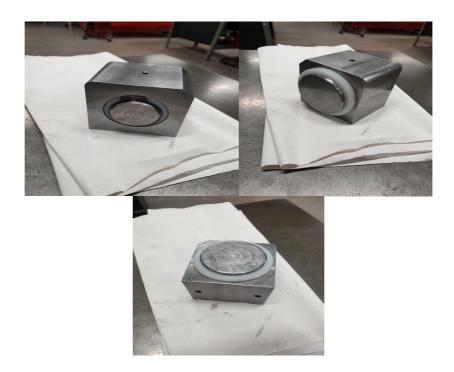
Photograph 32 - showing the completed bearing housing with minimal tool marks achieved.
