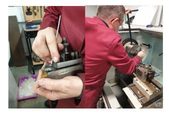
Photographs 25, 26 and 27 – showing the preparation of the CNC lathe. The program simulation was run to see the general outlook of the part. The program was then run but in tracking mode to start with to prove first pass. The program was then changed to CNC mode. Coolant was turned on and part run with the 4 tools being changed at the right time.
