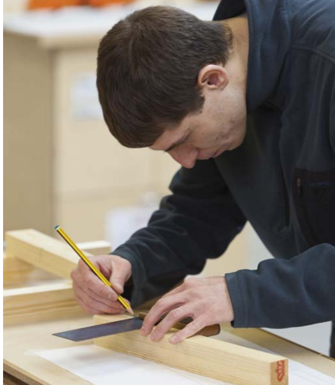
Marking out a mortice
