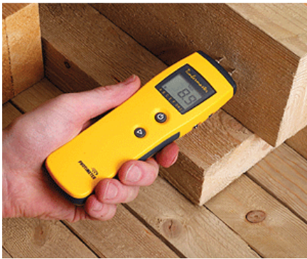
Moisture meters are used to measure moisture in timber
