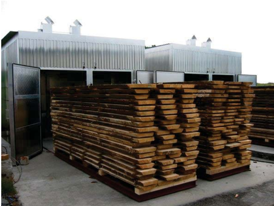
A kiln oven used for drying
