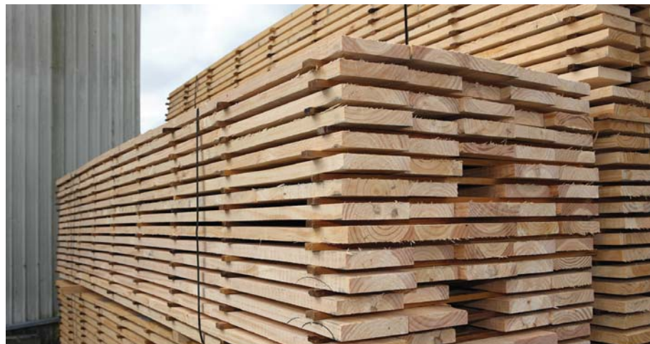
Incorrect storage – timber should be stored in the dry and away from UV
