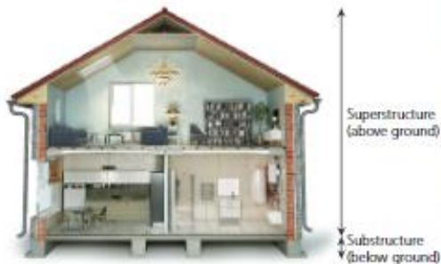
▲ Figure 3.1 Superstructure and substructure of a building
