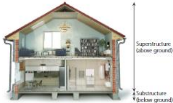
▲ Figure 3.1 Superstructure and substructure of a building
