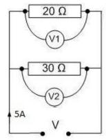
For the circuit shown, what would be the voltage reading of voltmeter (V1)?
