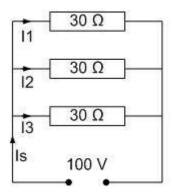
What is the power dissipated in the circuit shown?
