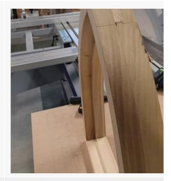
Loose tenon with small gap not exceeding 1mm
