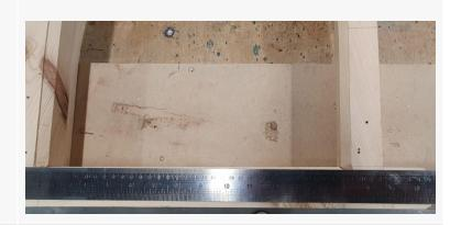
Mitre to rebated mortice and tenon tight within 3mm. Chip on shoulder, not scribed. Pen used for marking out rather than pencil.
