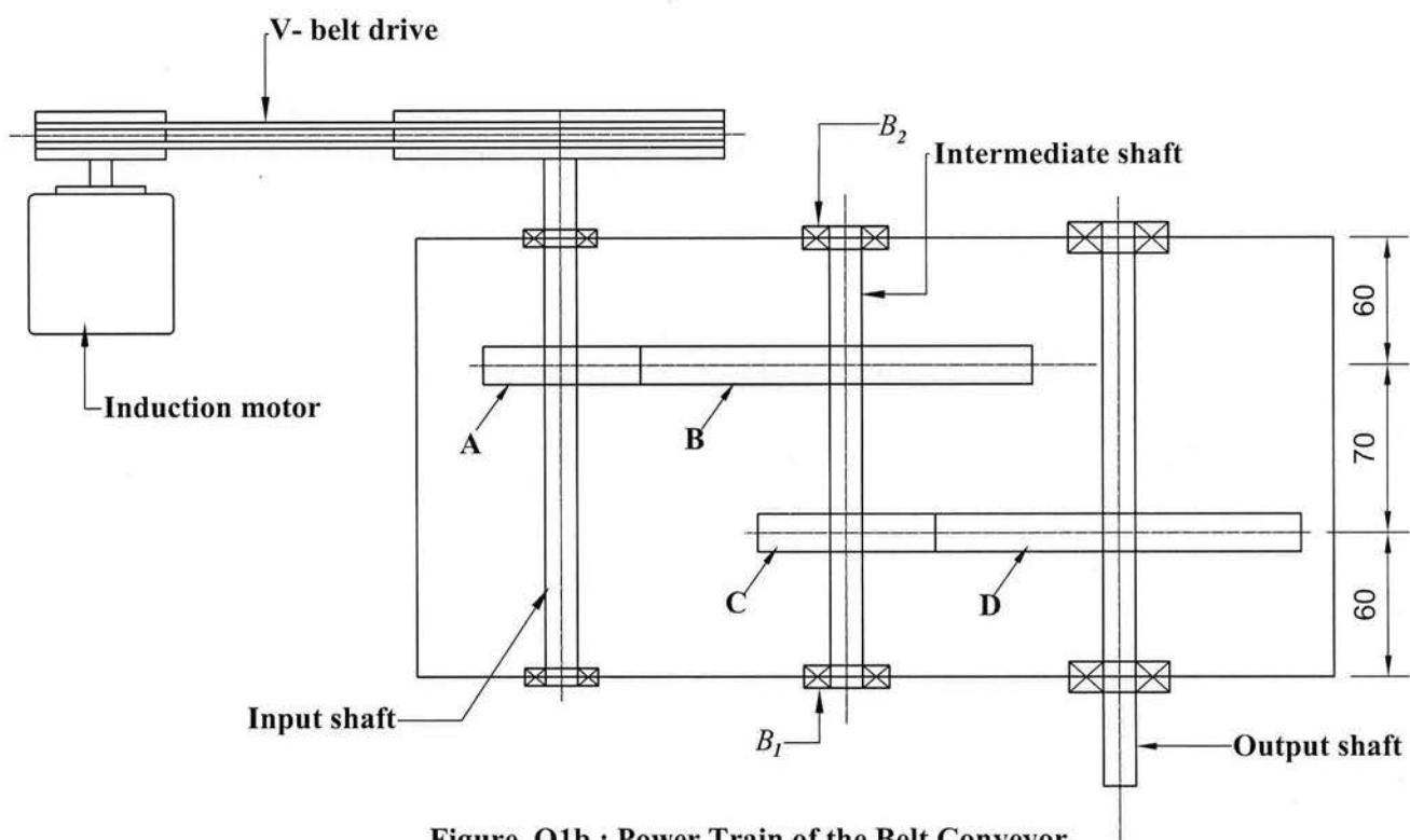
**Figure Q1b : Power Train of the Belt Conveyor**
