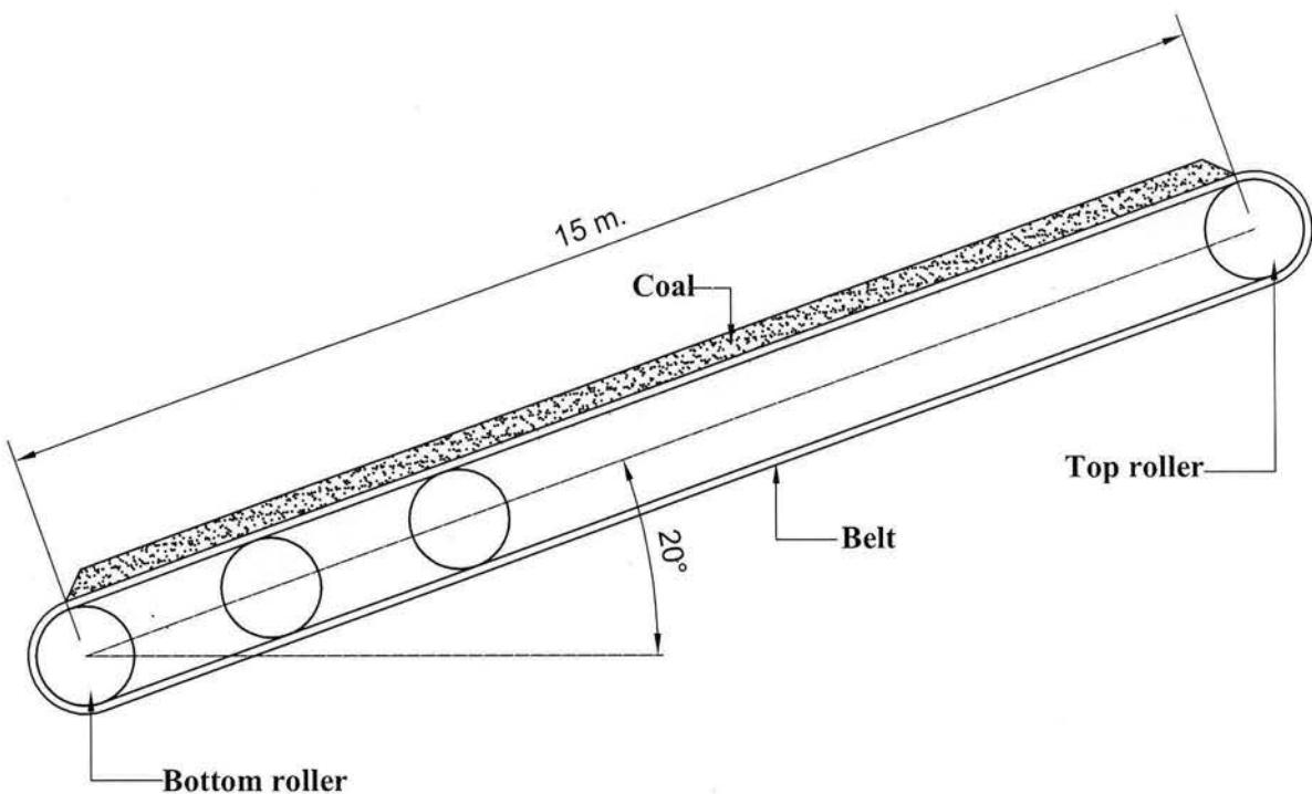
**Figure Q1a : Schematic Diagram of the Belt Conveyor**
