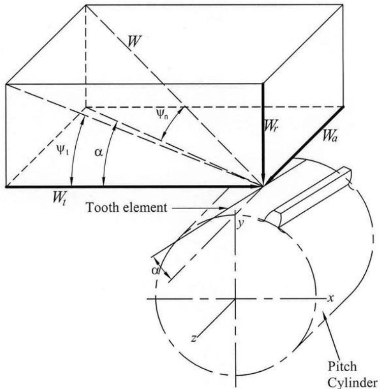
$W_t$  - tangential tooth load on a transverse plane
