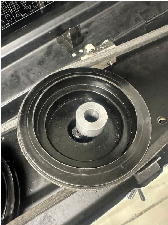
this is the pulley without any form of bearings in.
