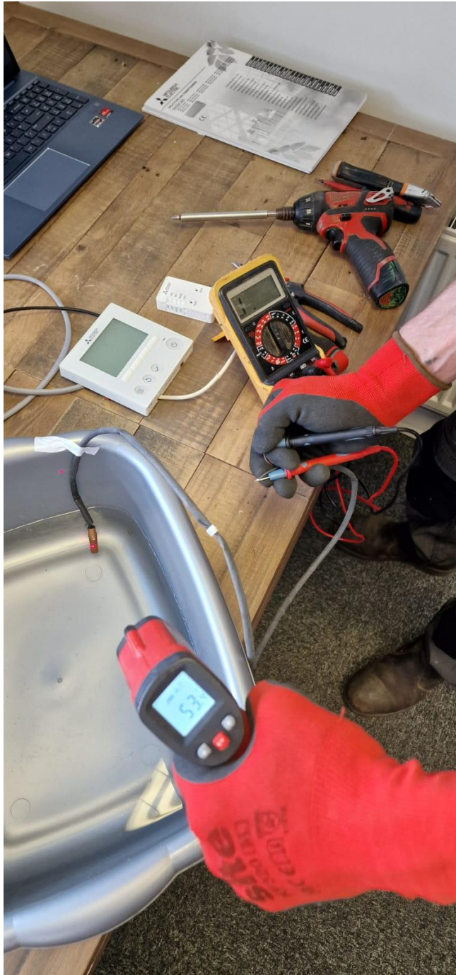
Photographs 3 and 4: Photographic evidence shows the test set up for the calibration including displays of test equipment showing the simulated temperature and the values obtained.
