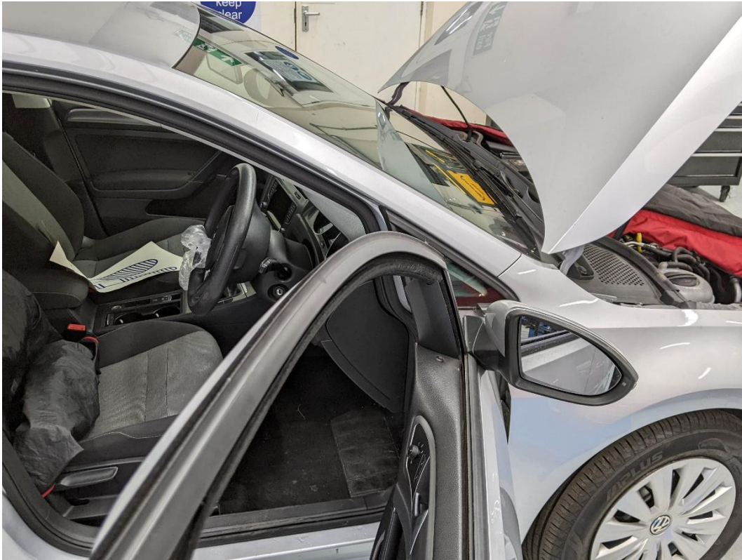
Photograph 2: Photographic evidence shows the prepared and not fully accurately fitted VPE. Steering wheel cover has mostly come off, the foot well protection is on the passenger seat rather than the driver's side floor and the seat cover has also partially come off from the seat. Wing cover has moved to under the bonnet instead of the wing.
