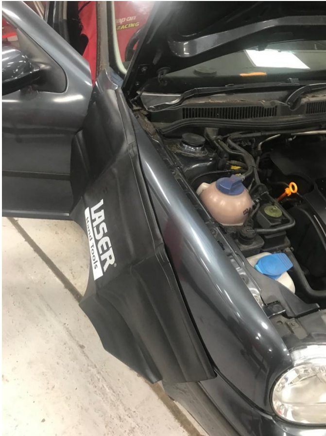
Photograph 2: Photographic evidence shows the prepared but not fully accurately fitted VPE on Vehicle 1, the wing cover is noted as sliding off.
