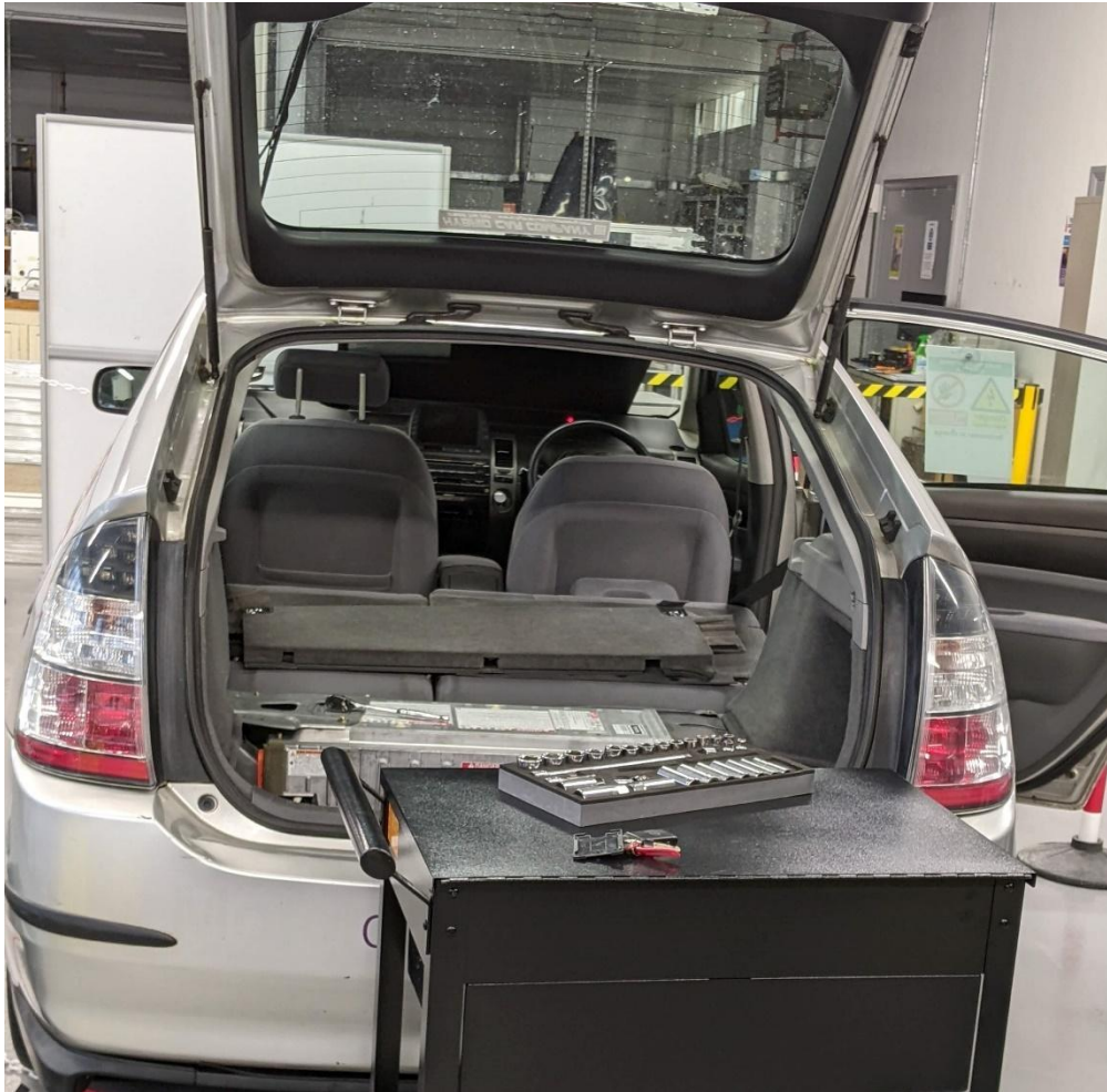
Photograph 3: Photographic evidence shows the high voltage battery correctly exposed with tools prepared but placed improperly.
