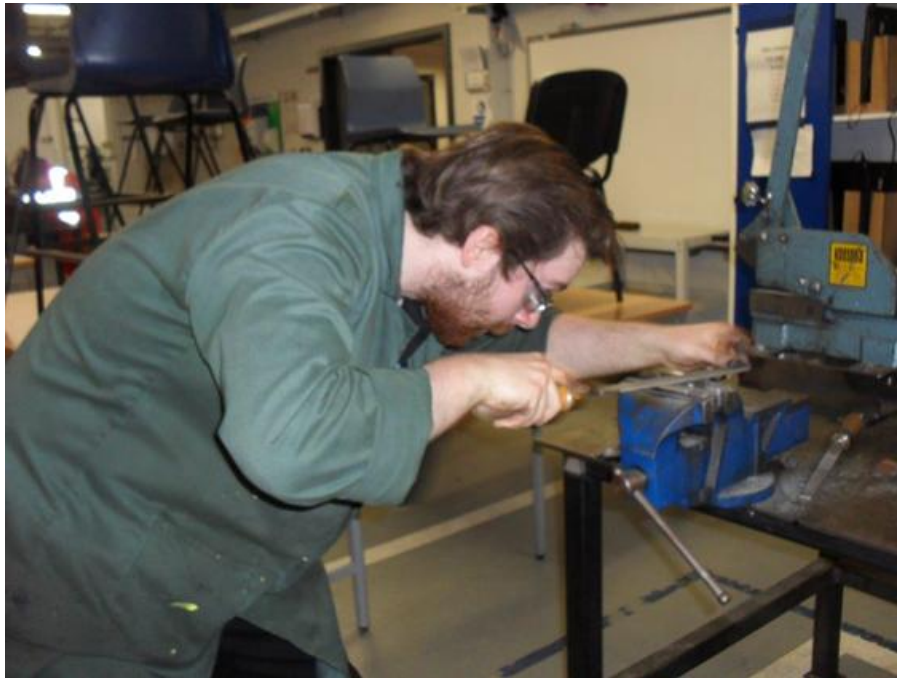
Photograph 3 – showing the datums being established using a file.
