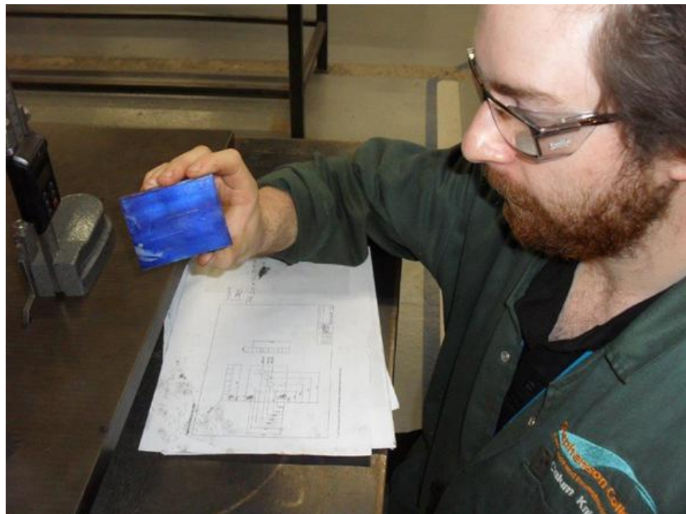
Photograph 4 - showing the preparation of the material, engineer's blue has been neatly applied even to the stock.
