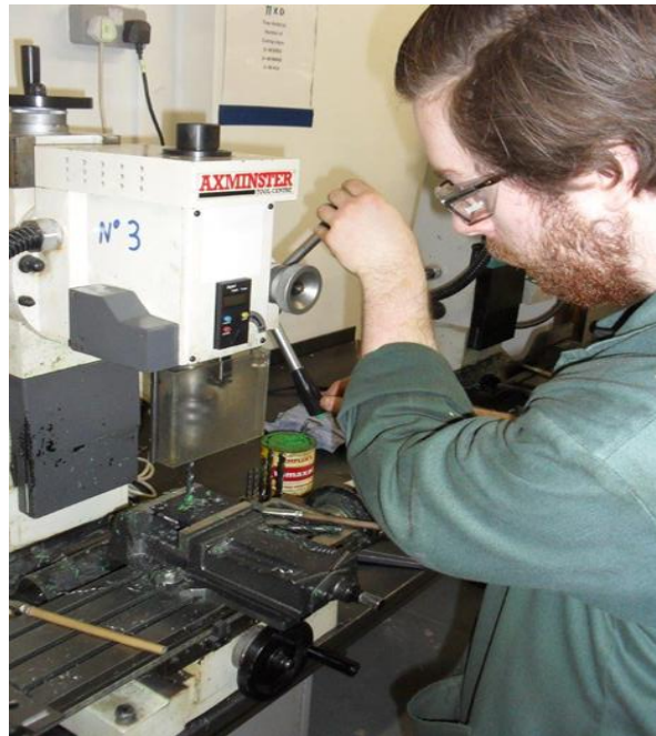
Photograph 8 – showing the safe use of equipment, with the pillar drill operated using correct PPE and with all guarding in place.
