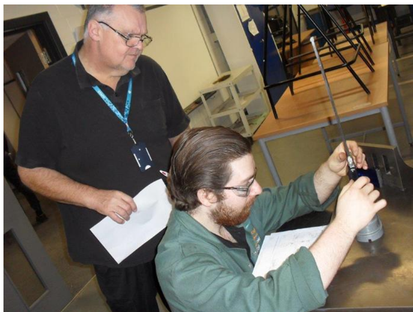
Photograph 9 – showing the correct use of a Vernier height gauge whilst performing in-production checks.
