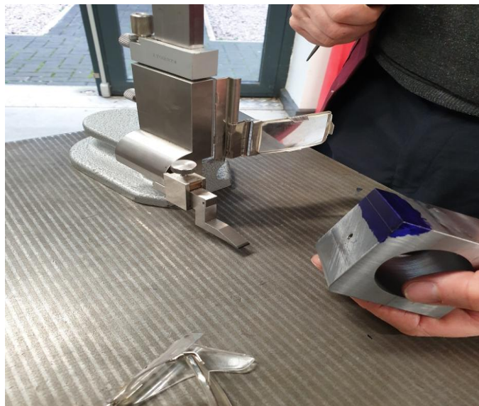
Photograph 10 - showing 8mm chamfer blued and marked with the vernier height gauge.
