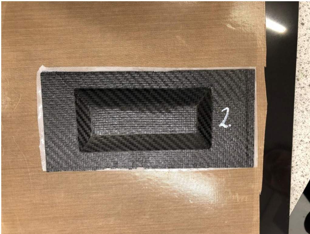
Photograph 36 – showing the spacer block component placed on top of release film.
