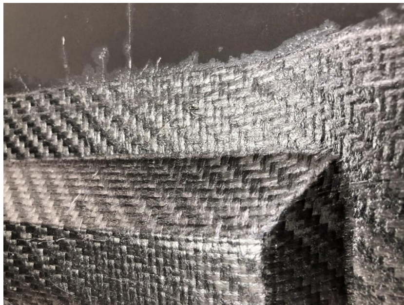
Photograph 27 – showing detail of edges, corners and transitions showing good definition and orientation of fibre.
