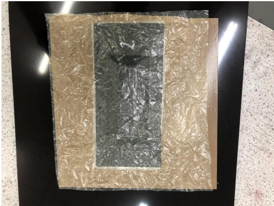
Photograph 37 – showing release film placed on top of the moulding. Note: the release film is sufficiently wrinkled to aid draping.
