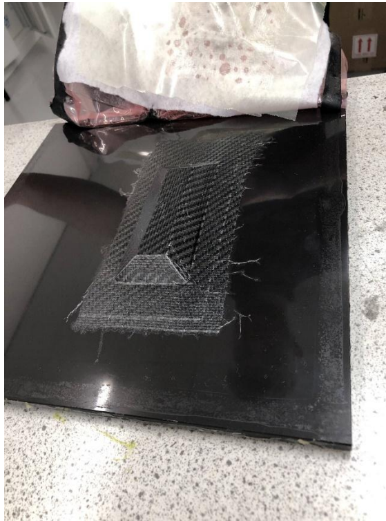
Photograph 26 – showing the release film being removed and moulding is further inspected.
