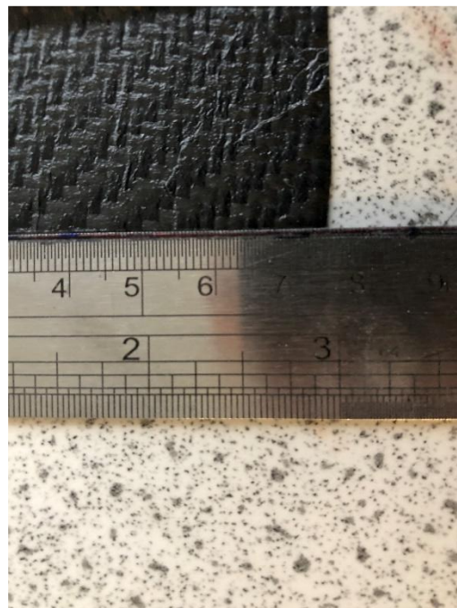
Photograph 47 – showing candidate checking straightness of short edge. Note: the tapering of the edge and lack of straightness.
