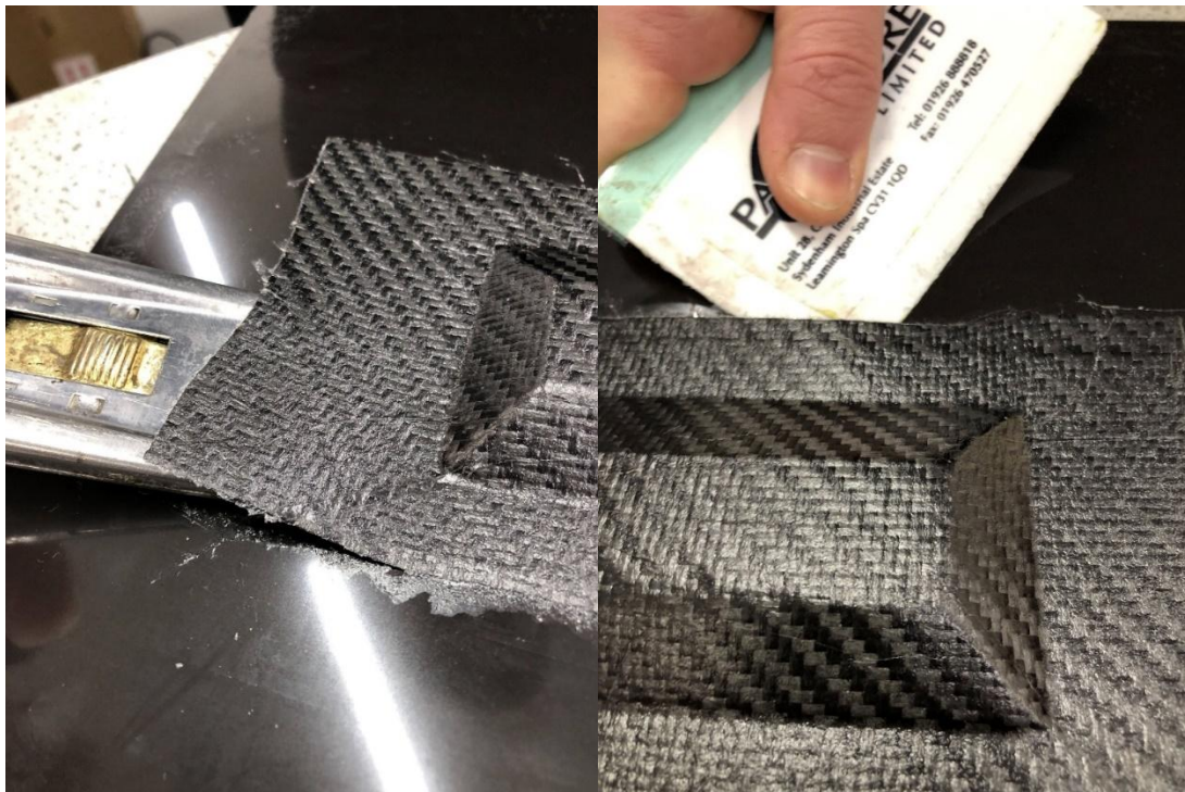
Photographs 25 and 26 – showing a scraper being used to lift one corner at the beginning of the demoulding, followed by a plastic wedge to complete the process of demoulding, ensuring that the lift is not too abrupt to overstress or crack the laminate.
