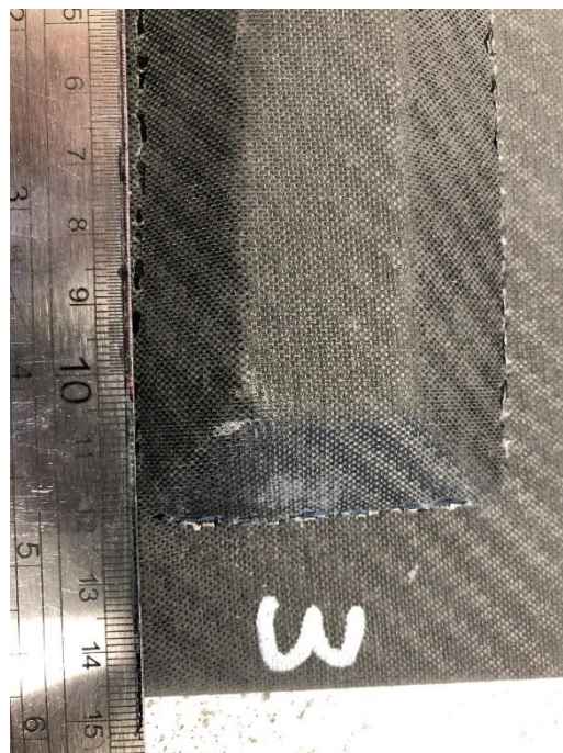
Photograph 45 – showing candidate checking straightness of long core length dimension.
