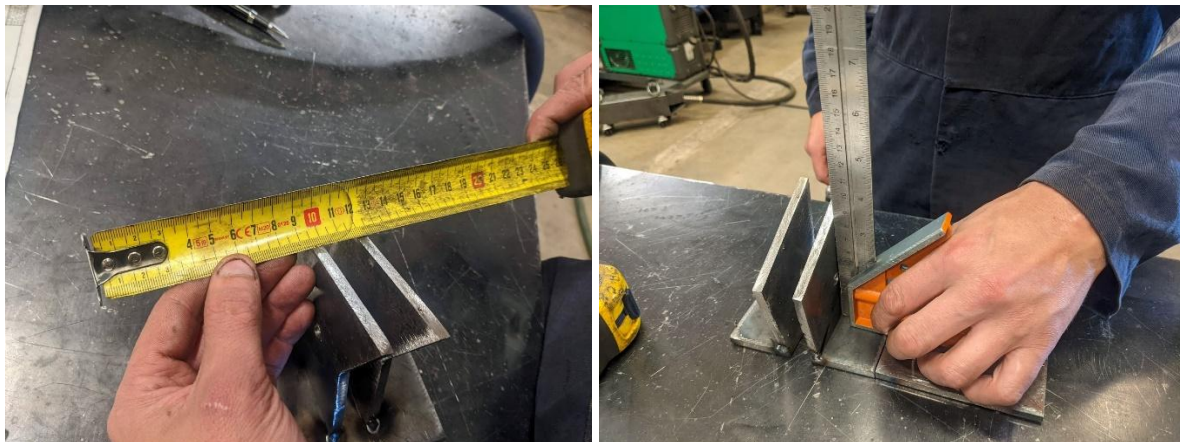
Photographs 15 and 16 – showing the candidate carrying out in-production checks to ensure the components have been welded square and are at the correct size.
