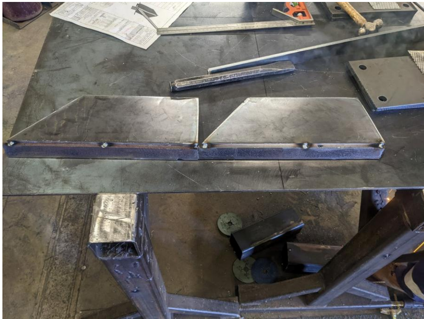
Photograph 18 – showing the crown welds. Note the straight bead on the left and the uneven bead on the right.
