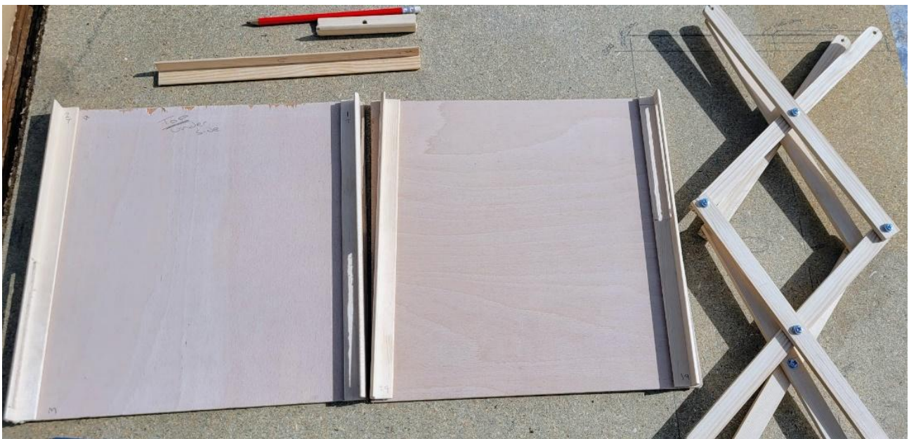
Photographs 4 and 5 show the markings and the assembly process of the prototype using a rod board for accuracy. The holes have now been cut out of the rails and they are neat and well aligned.
