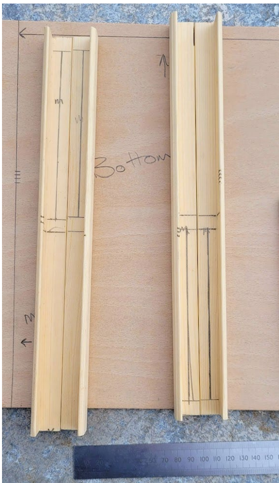
Photograph 3 shows the sides for the runner rails marked up. The lengths of the rails are not accurately cut (negotiable +/- 1-2 mm). The markings for the holes for the runners are missing and the level of detail is limited.
