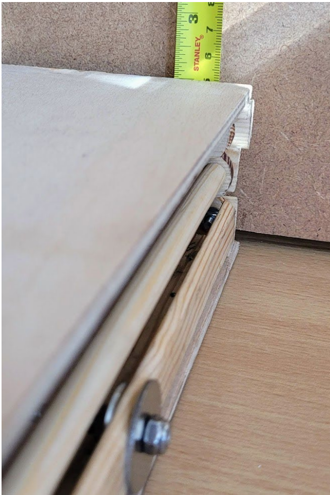
Photograph 7 shows the lifting platform at its lowest height of 50 mm, which meets the scaled dimensions required.
