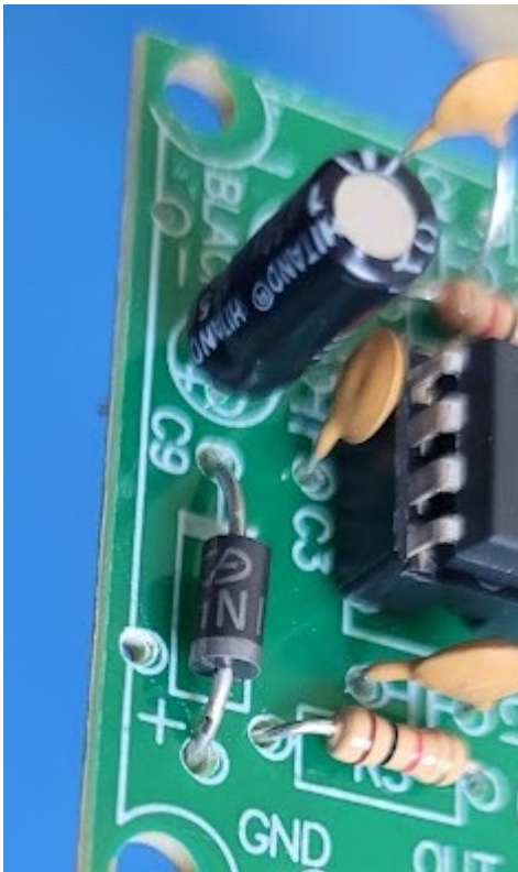
Photograph 10 shows that the diode is fitted the wrong way round, with the wrong polarity. The candidate spotted and corrected this mistake as they progressed with the construction.
