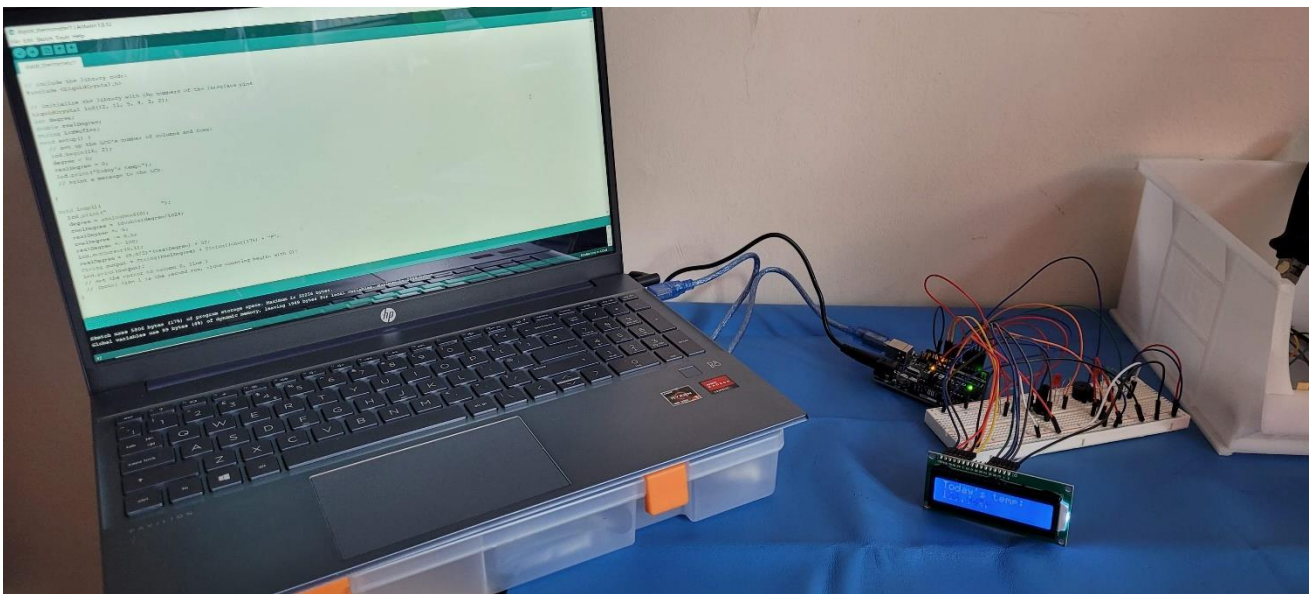
Photograph 6 shows the positioning of the sub-assemblies. Ordering is accurate and functional. The Arduino coding program is running and the correct connections/interface to the laptop have been used. The coding is accurate for correct operation of the system. The system is laid out to prevent accidental dislodging of wires or components.
