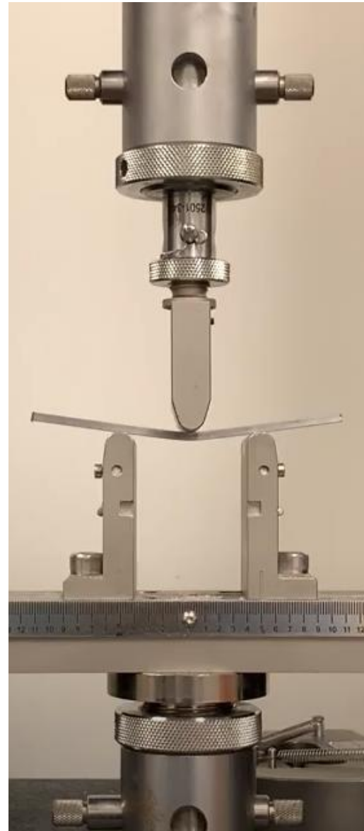
Photographs show the process used for the three point bending test on bar. The left image has the test piece in place, the middle image shows force being applied to the test piece and the right image shows the stress point has been met and the material has folded.
