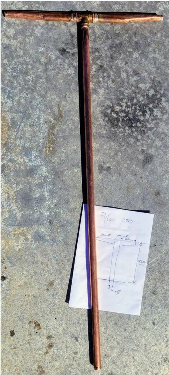
Photographs 6 and 7 show the completed soldered joins, demonstrating the taper of the arms, the cable fixing points, with insulation and base.
