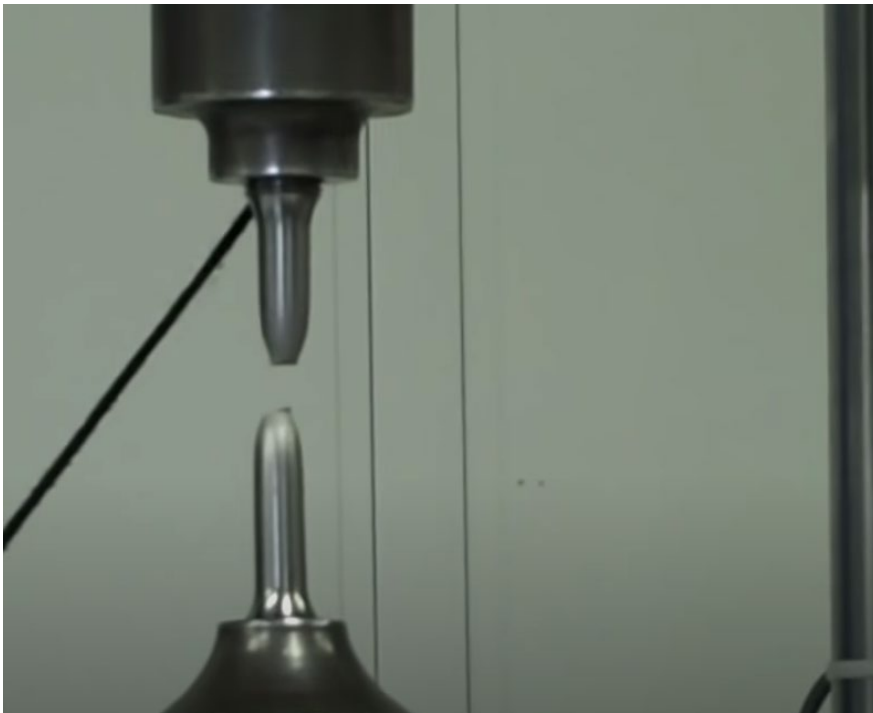
Test piece fractured after Young's modulus has been met.
