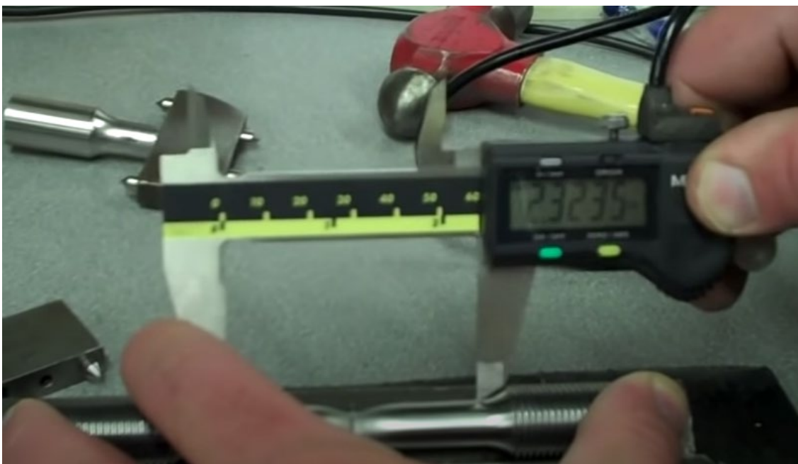
Measuring to determine and prove fracture location, this can then be scaled to an approximate location on the pylon.
