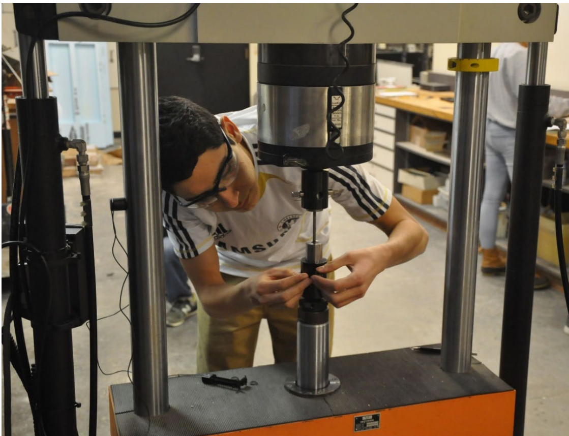
Candidate setting up the tensile testing machine with the appropriate PPE.
