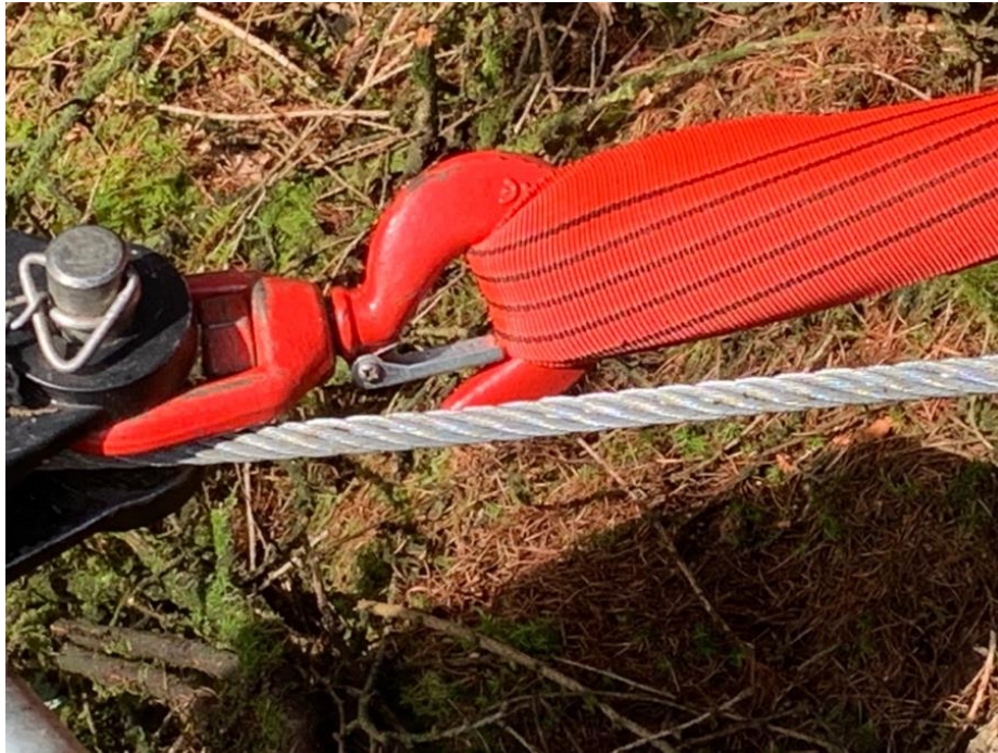
Above: Winch connected directly to sling with no shackle
