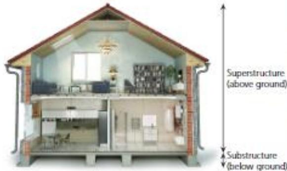
▲ Figure 3.1 Superstructure and substructure of a building
