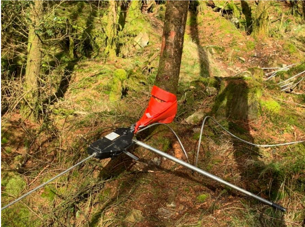
Above & below: winch connected to sling using shackle.
