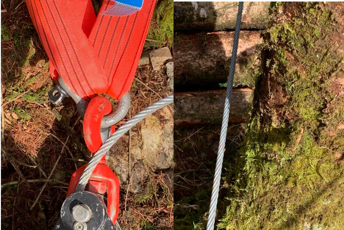
Above right: cable route free of obstructions.
